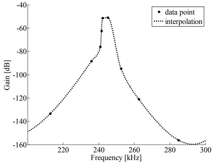
Figure 2. Illustration of the frequency response of the used PWAS (D-9.55mm-1.00mm-850 WFB, APC International)
