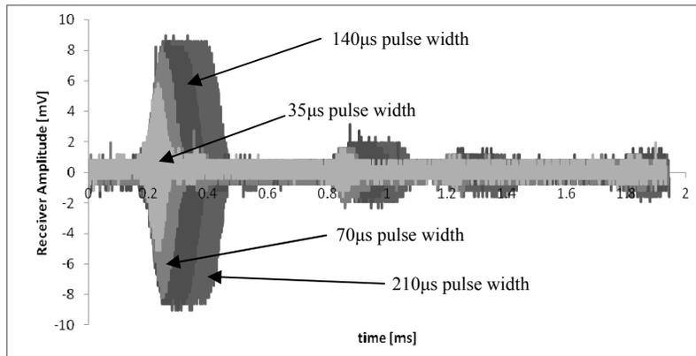
Figure 3. Illustration of received signal strength with a different transmitter pulse widths
