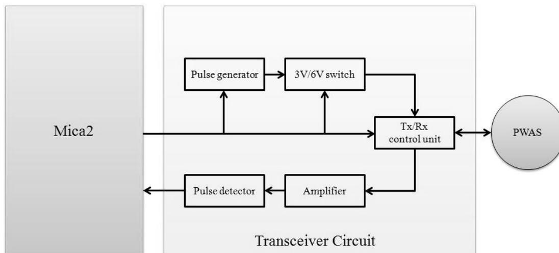
Figure 1. Block diagram of the ultrasonic pulse switching hardware platform
