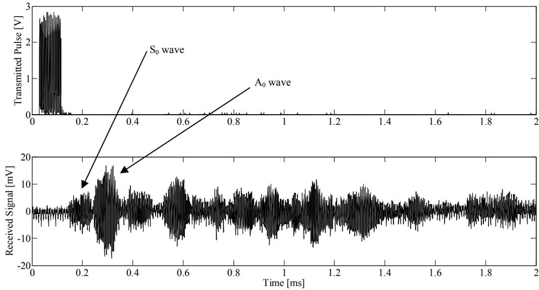
Figure 4. Transmitted and received signals at a distance of 1 meter
