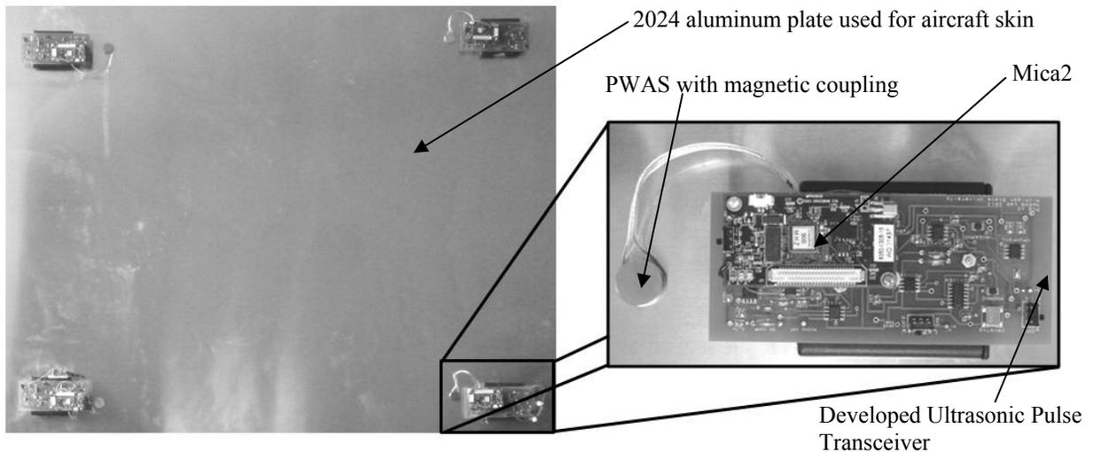
Figure 5. Illustration of multiple nodes mounted on the structure along with a detailed image of one hardware platform
