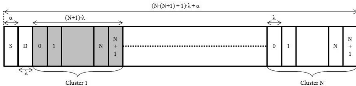
Figure 7. Introduction of the frame structure for  $N$  nodes in a WSN using mechanical wave propagation through solid substrates
